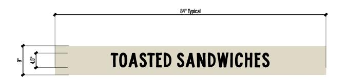
High resolution printed graphic bars (printed in revers on 3M™ High performance clear vinyl)
